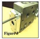
3. Apply one (1) drop of Blue Loctite (removable) to exposed threads of Cylinder Coupler as shown
