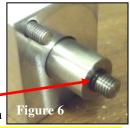
in Figure 6. Note: Insure that O-Ring is in groove by shoulder.
