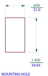
PANEL THICKNESS (SNAP - IN BRACKET) .030 MIN --- .187 MAX
