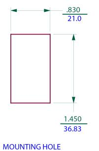
PANEL THICKNESS (SNAP - IN BRACKET) .030 MIN --- .187 MAX .76 4.75
